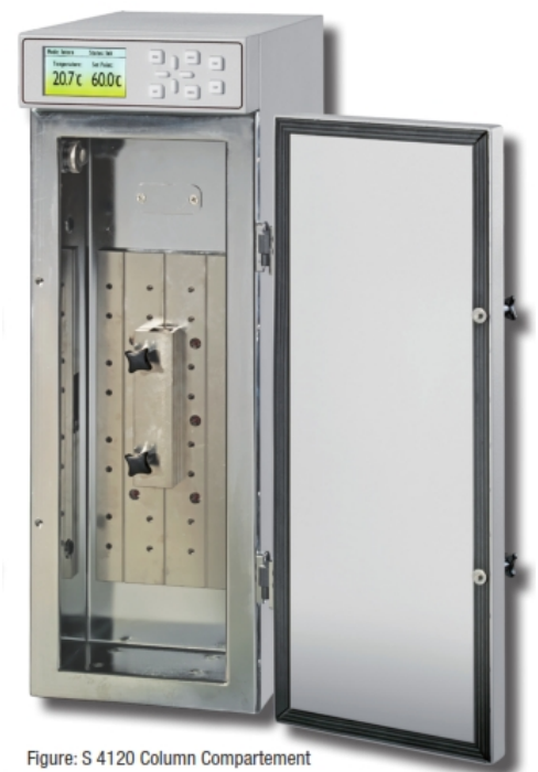
Figure: S 4120 Column Compartment
